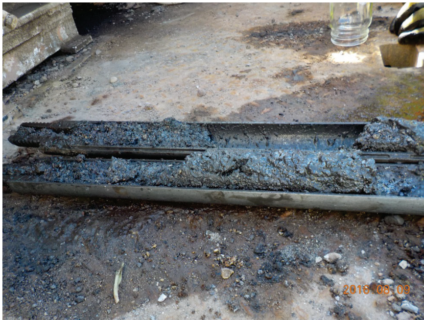
Boring B-23 Date: 8/9/16 Depth: 24' – 26' Notes: Slight naphthalene odor with a slight sheen.
