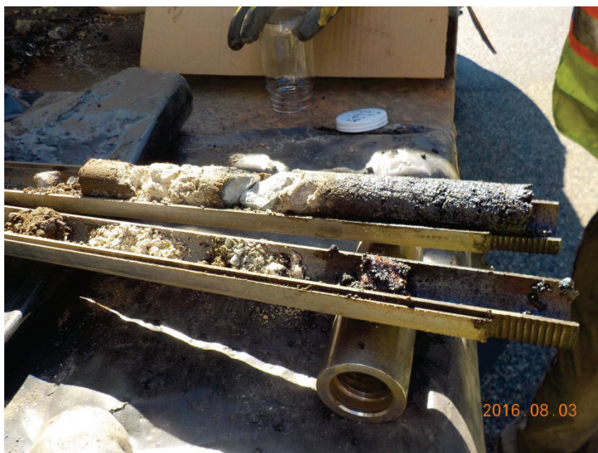
Boring B-14 Date: 8/3/16 Depth: 10' – 12' Notes: Moderate naphthalene odor with very slight sheen.
