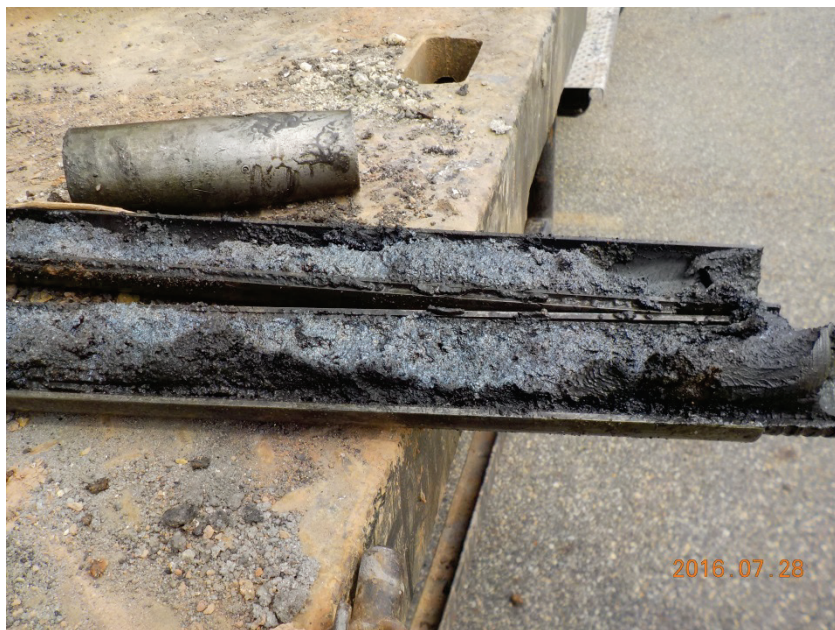
Boring B-5 Date: 7/28/16 Depth: 24' – 26' Notes: Slight naphthalene odor with moderate sheen.
